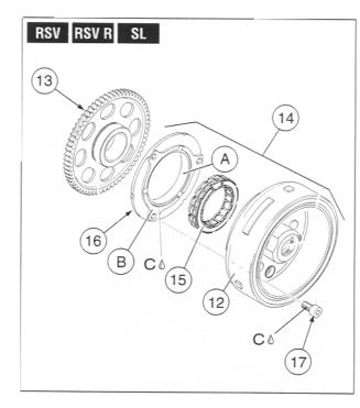
◆ Correctly insert the sprag clutch (15) in its seat, on the sprag clutch flange (16). Refer to the reference dot (C) applied during disassembly.
